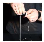
The height is also adjusted using this joint. With the single cross laser, this can be done very easily by loosening the knurled screw on the side of the rod until the desired height is reached and then tightening it hand-tight.
