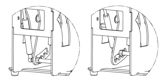
• Moving the contact point of the springs to the front lowers the closing force, while moving to
