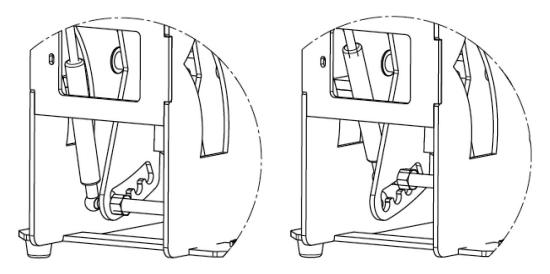
Moving the contact point of the springs to the front lowers the closing force, while moving to the rear increases it. Please note that sufficient force is required to ensure automatic opening of the press - the opening force decreases or increases along with the closing force.
