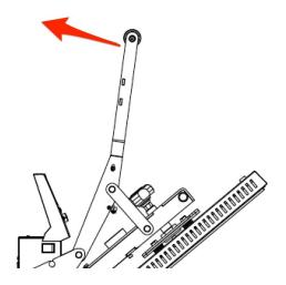
• In the released position, you can now access the connecting rod between the two gas compression springs from behind, lift it slightly and vary the position within the predetermined locking points. Caution! Danger of injury from trapping/crushing!
